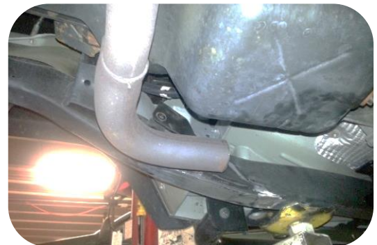
Figure 6 Exhaust after cutting
