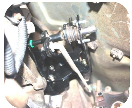
Figure 9 Transfer Case Linkage Installed
