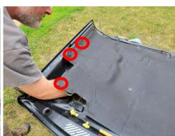
Remove the plastic vent by pressing on the 6 clips on the inside of the hood
