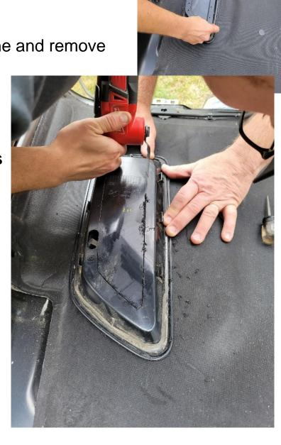
From the outside of the hood cut a slit in the liner to mark the location of the hole
