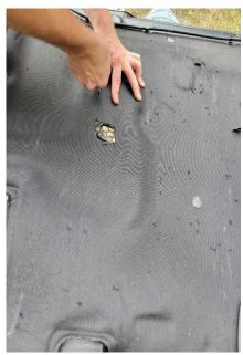
Line up the honeycomb part to the large hole now in the liner and cut out the outside contour of the part. Increasing the size of the hole in the liner. Do not cut out the channel on the side of the honeycomb part. Cut along the green line in the picture below.
