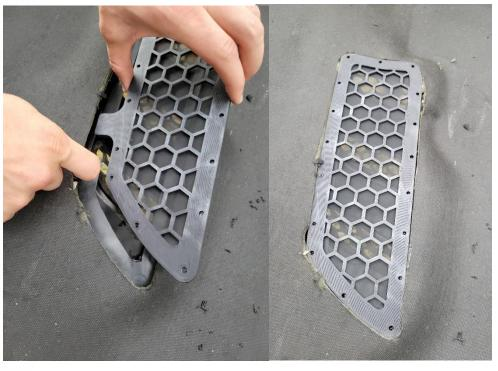
Start in the center of the part and work your way out gently tightening the screws with a washer as you go with a screwdriver
