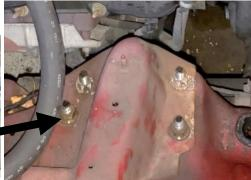
3. This will give you access to the nuts securing the strut assembly to the body. Do not loosen at this time.
