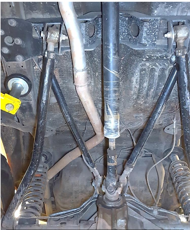
Recommended custom exhaust routing
